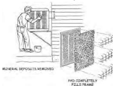
FIG. 4-18: COOLER PADS AND FRAMES
