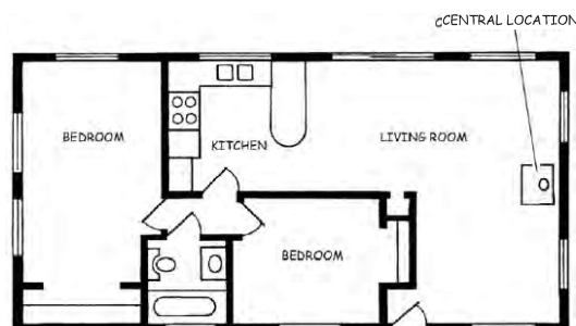
FIG. 4-27: WOOD STOVE/INSERT CENTRAL LOCATION
