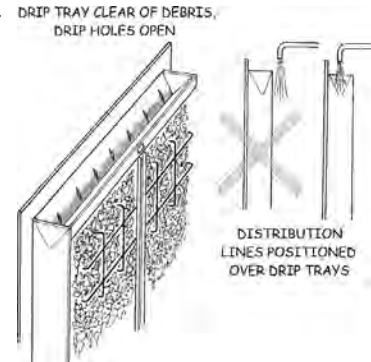
FIG. 4-20: WATER DISTRIBUTION TO DRIP TRAYS
