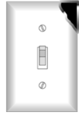
CRACKED OR BROKEN COVER PLATE Graphic Credit: RHA, Inc.
